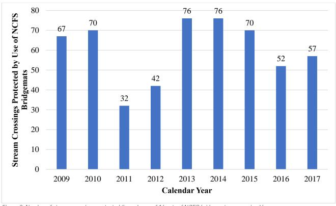
Figure 8: Number of stream crossings protected through use of 16 sets of NCFS bridgemats summarized by year.
