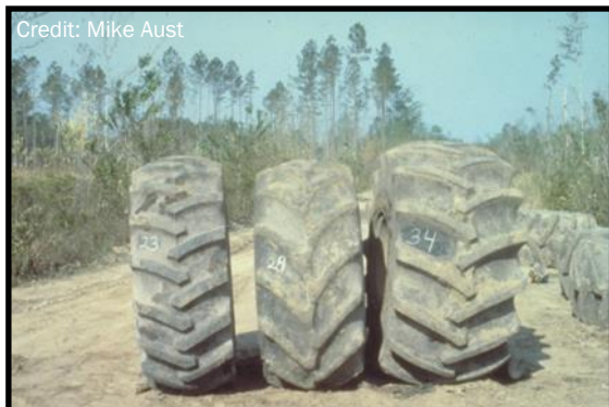
Skidder tire selection, sizes 23, 28 and 34-inch wide (left). Dual-tired skidder using a bridgemat stream crossing (right).
