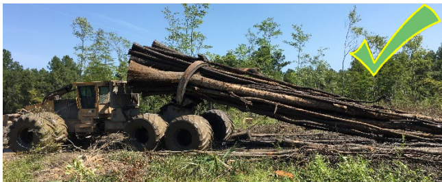
Side view of a skidder running atop of a shovel skid trail.
