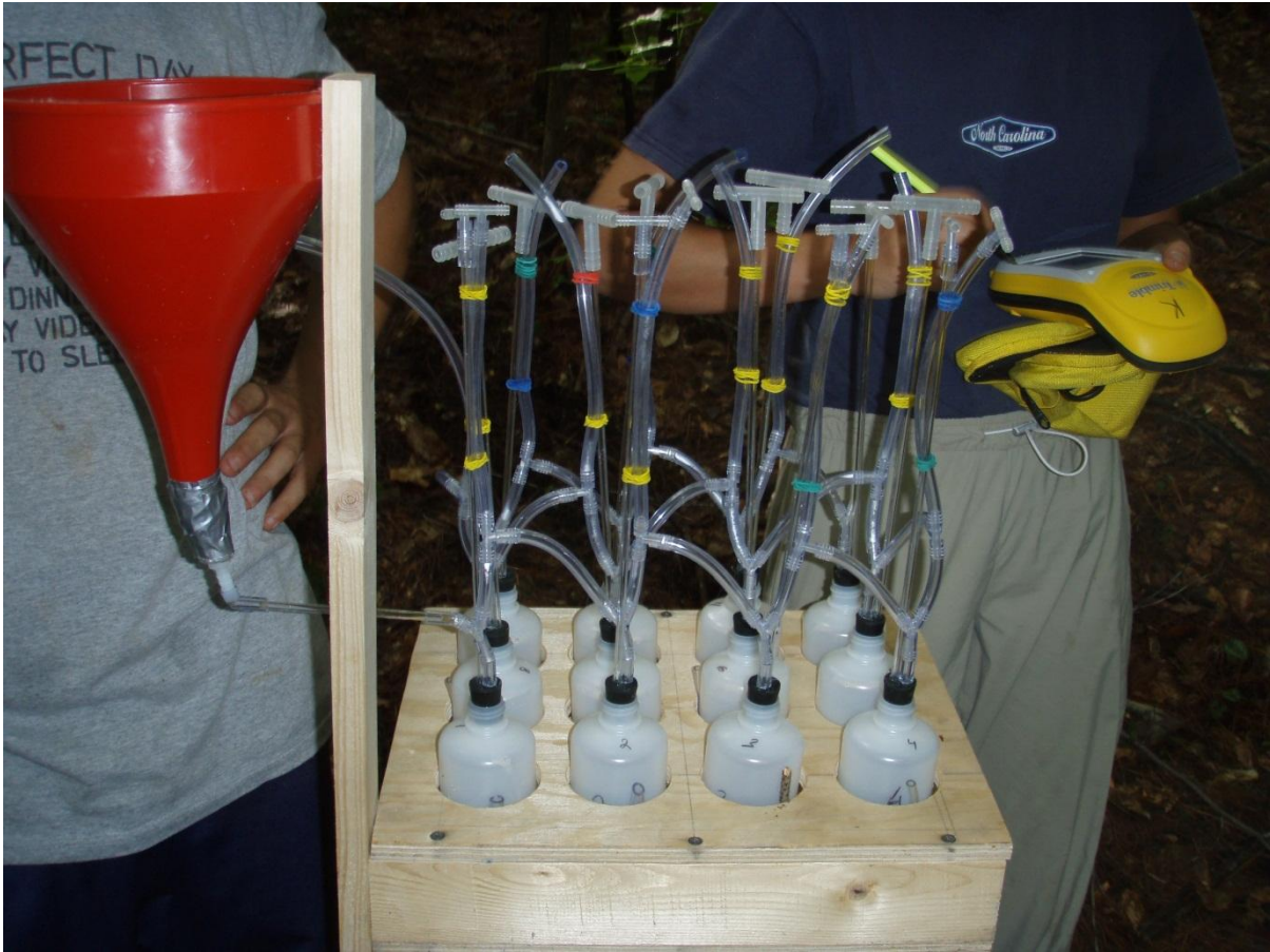
Figure 20. Sequential rain sampler built and laboratory tested prior to field installation by Y. Kuntukova.
