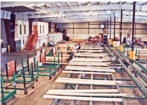
Figure 3. At the hardwood sawmill's "green chain," processed lumber is classified into grades and lengths, and sorted accordingly. Photo credit: Robert Smith.
