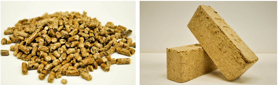
Figure 8. Wood pellets (left) and wood briquettes (right). Photo credits: Maria Fernanda Laguarda Mallo.
