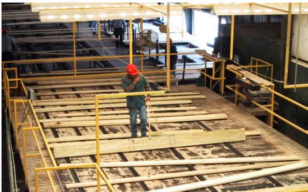
Figure 4. A grade inspector grades lumber as it travels on a hardwood sawmill conveyor. Photo credit: Phillip Araman.
