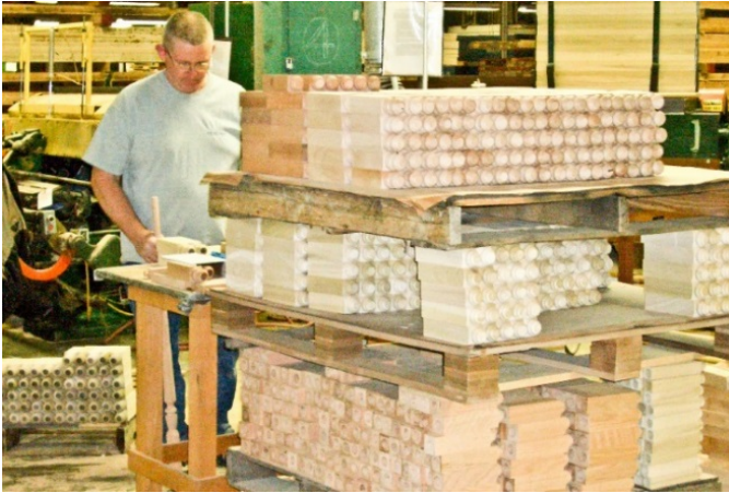
Figure 22. In stair parts manufacturing, transformation takes place in different machining centers, such as “gluing” and “turning.” Photo credit: Omar Espinoza.
