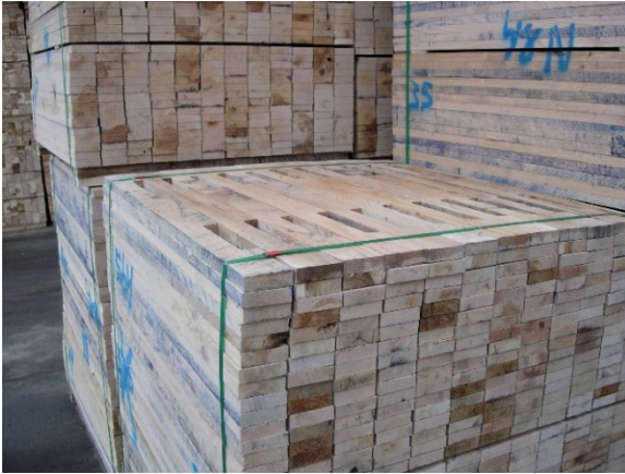
Figure 11. Pallet stock, usually produced from interior portions of higher grade saw logs. Photo credit: Brian Perkins.
