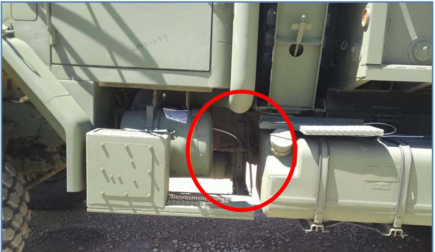
The airline manifold—located under the driver's door—is circled in red. (This is a truck/engine similar to the one involved in this incident.)
