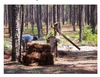
**Building Your Box-Baler:** Constructing a box baler is as simple as building and securing a crate upon a wheeled platform. Whether you build the baler from new or used parts, you'll need larger tires on the rear to be able to maneuver over logs and brush. The front wheels are optional and most balers use fixed feet which provide a stable base for compacting the straw into a tight bale.
