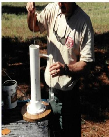
Figure 3. The water displacement method was used to determine cone specific gravity. Specific gravity was determined within five minutes of collection.
